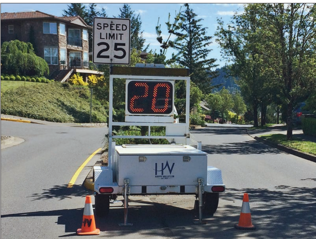
The City's radar trailer helps Happy Valley gather useful traffic information. This compact piece of equipment can be set up wherever traffic concerns arise
