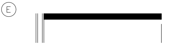
LOCATE STOP BARS PER ODOT STANDARD DRAWING TM530. 12" STOP BAR
