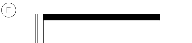
LOCATE STOP BARS PER ODOT STANDARD DRAWING TM530. 12" STOP BAR
