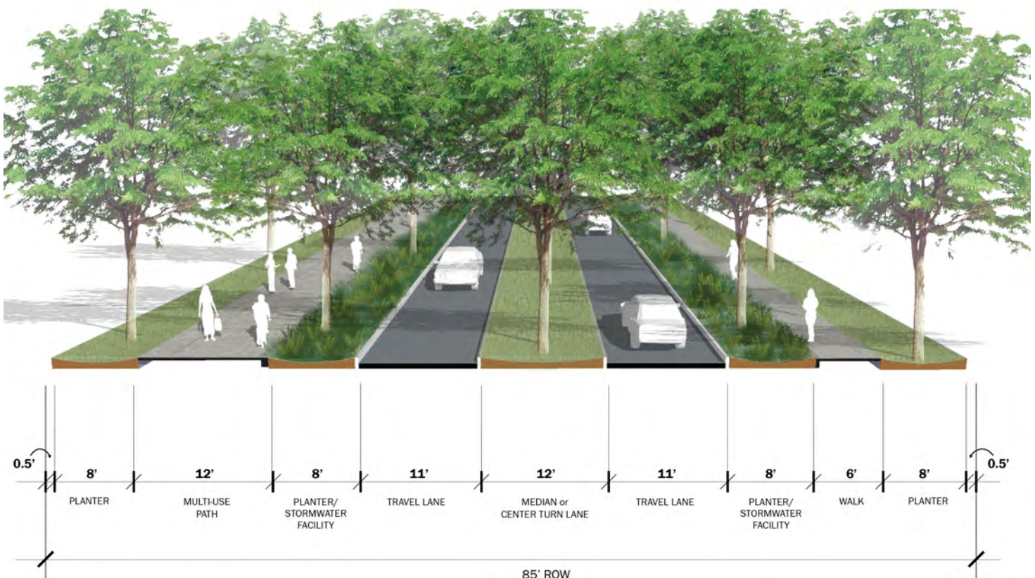
Figure 19. Recommended Foster Road Cross-Section (Looking North)
