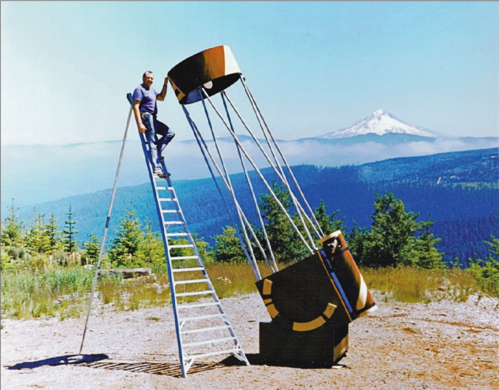
Steve Swayze shows off an approximately 800-pound telescope he built with a 40-inch mirror near Mount Hood.
