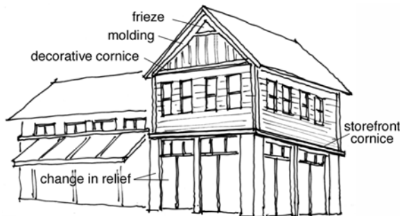
This sketch shows an example of a well articulated building façade featuring elements such as awnings, storefront windows, and varying materials to create interest.
