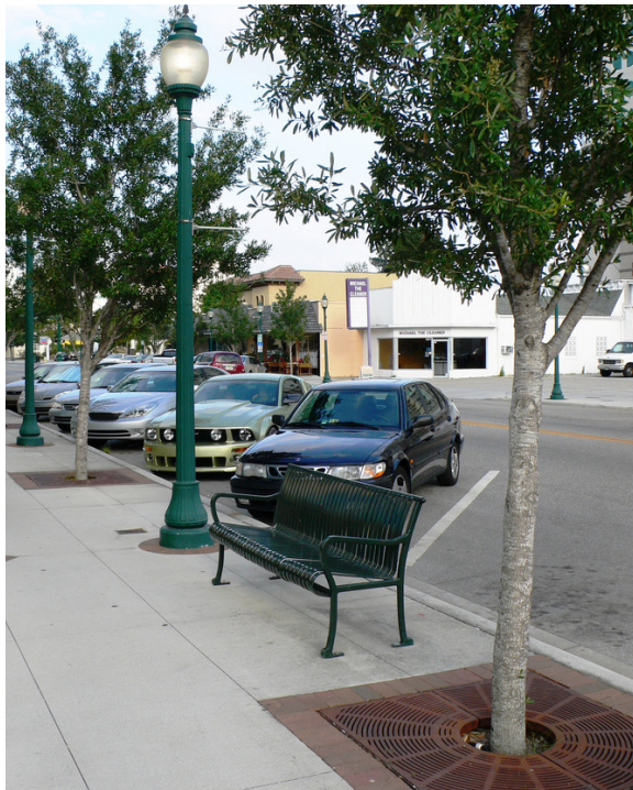
Tree grates, benches and street lights are basic elements in creating a pedestrian friendly streetscape. The selection of light fixtures to provide adequate lighting without glare is crucial, as is the selection of tree species to maintain visibility of storefronts and minimize maintenance.
