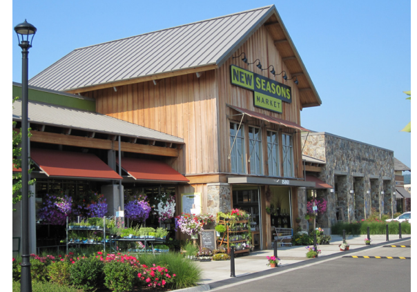
This local grocery store employs a dramatic change in the roofline to support complex massing and emphasize the building's main entrance.
