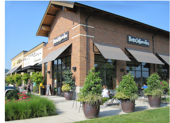
This Happy Valley building uses a taller pitched roof to emphasize the street facing corner of the development. While the entire structure is single-story, the change in the roofline provides a visual emphasis.
