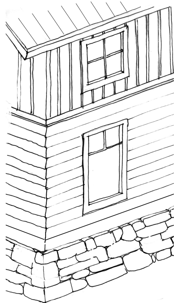
Multiple materials may be incorporated into a single building, with the heavier materials at the base and lighter materials above.
