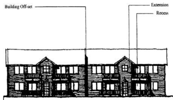
Figure 16.44.010-F Example of Extensions and Recesses
